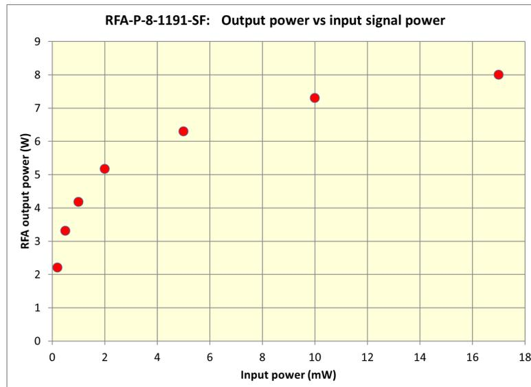
Fig. 4. RFA output power as a function of the seed input power.
