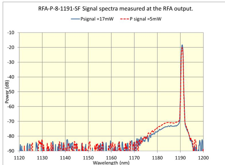
Fig. 5. Output spectra of at the output of 8-W 1191-nm RFA measured with 0.5-nm resolution when the seed input power was set to 5 mW and 17 mW. The Signal-to-ASE ratio is 50 dB and 55 dB, respectively.
