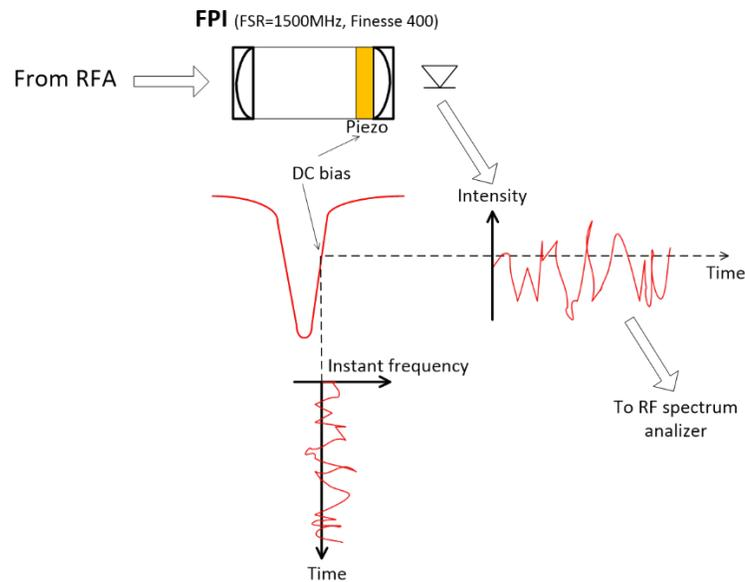
Fig. 9. Frequency noise measurement set-up.
