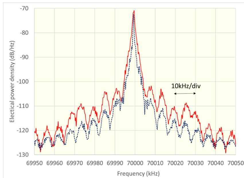
Fig. 12. Beat note measured after 35km unbalanced interferometer before and after amplification.
